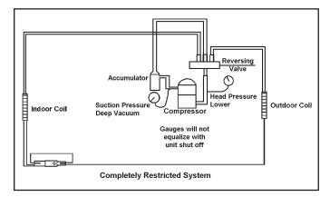
Restricted refrigerant systems display the same symptoms as a "low-charge condition." When the unit is shut off, the gauges may equalize very slowly. Gauges connected to a completely restricted system will run in a deep vacuum. When the unit is shut off, the gauges will not equalize at all.
